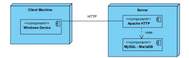
DAOS requires an internet connection in order to connect to the database. Client machine will interact with the server using HTTP requests. When a user opens the program on their computer it will be connected to the MySQL database which is in Apache server.
