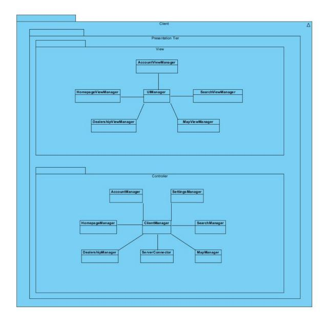
The client corresponds to the desktop application of our system. The client is the presentation layer of our system. The user creates an account or logins to the system
